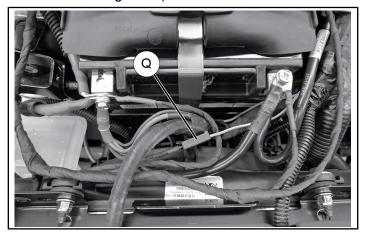
5. Route LED connection over to matching light bar connection. Location ® may vary depending on lighting accessory installed. Approximate location shown below for reference.
