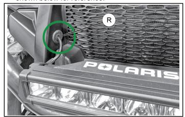
6. Secure all wires in place using cable ties.
