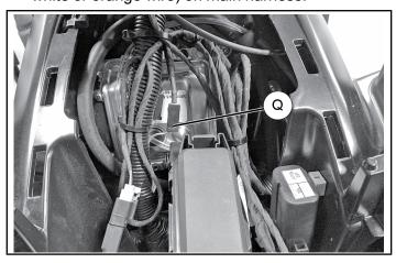
5. Route LED connection over to matching light bar connection. Location ® may vary depending on lighting accessory installed. Approximate location shown below for reference.
