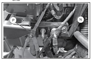
4. Join the male keyed power terminal (orange/white strip) ①, to matching female terminal (orange/white or orange wire) on main harness.
